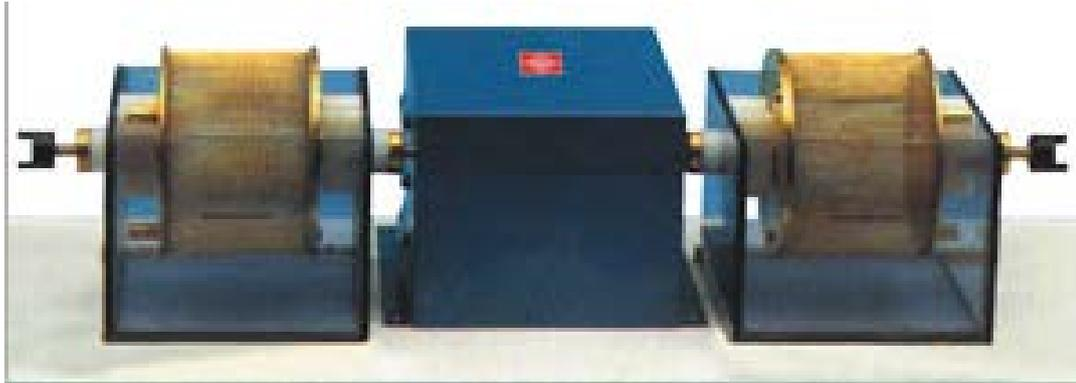
**Figure 2.5: Slake durability apparatus**
